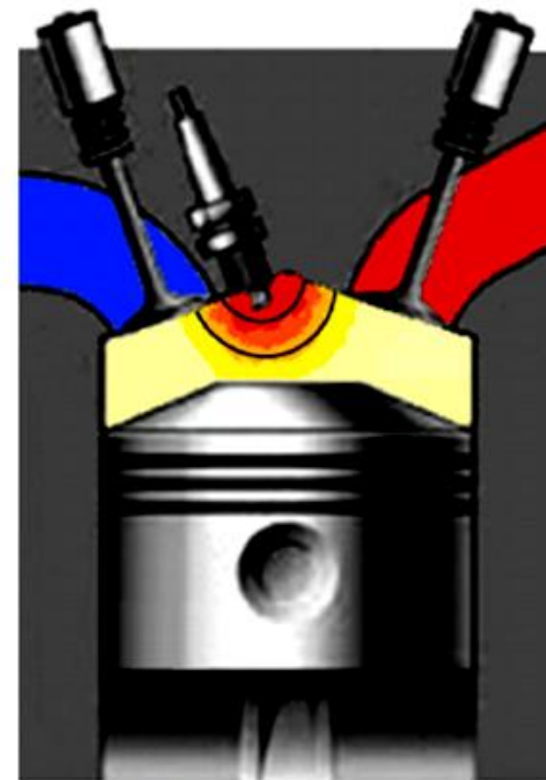
(b) Flame propagation.
