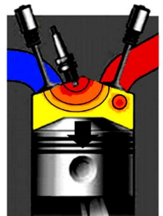
(c) Auto-ignition ahead of the flame.
