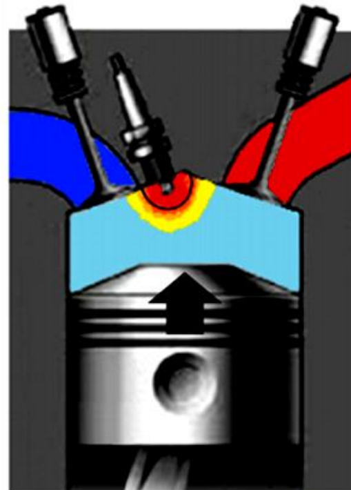
(a) Ignition by the spark-plug.
